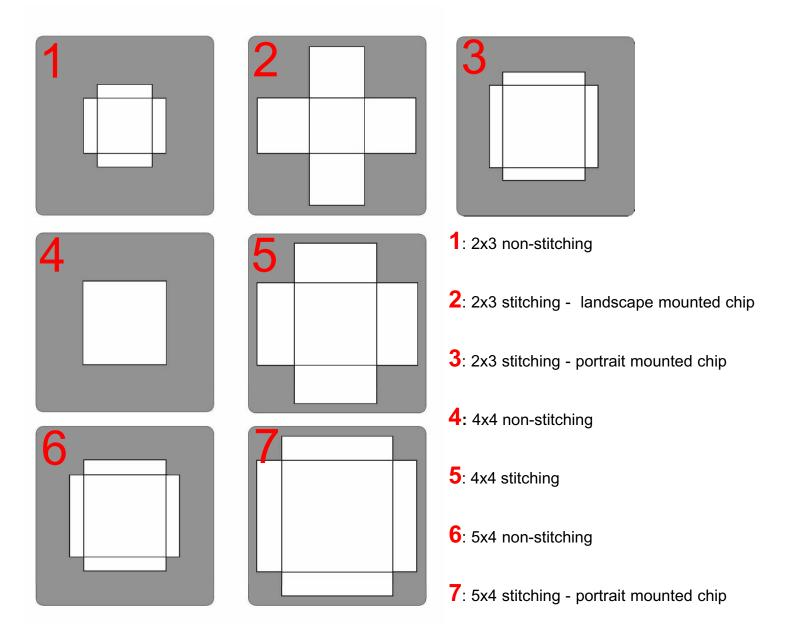
**Please note:** Most digital backs have 2 sets of Hasselblad mounting clips. This allows the back to mounted in either the portrait or landscape orientation. Landscape mounted chips and portrait mounted chips refer to the digital back's orientation relative to the Hasselblad mounts on the Fuji Stitching Adapter.
